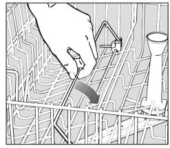
Place coffee mugs on top of the bar so that they sit at a slant. This allows all water to run off the base of the mug. The bar can also be used as a separator between two rows of glasses keeping them from leaning against each other. This protects the glasses and ensures good wash results. For wide items, flip the bar over to the right.
